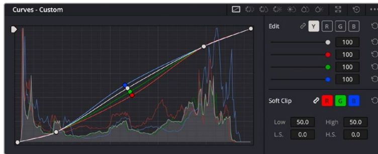
The curves palette is another tool you can use to make primary color corrections, or enhance specific areas of your clip when using a power window
