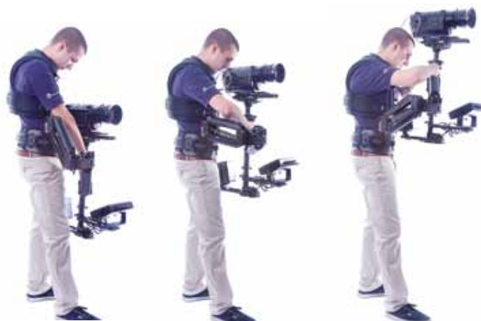
Boom the arm up and down, watching to see if the upper arm follows the forearm.
