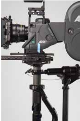
Camera c.g. .75" (19mm) behind center post – fore-aft.
