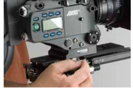
Closing the locking lever.
