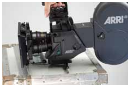
Finding the camera's fore-aft center of gravity.
