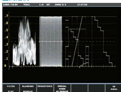
4 inputs Waveform parade Display (LV 58SER01A ×2装着時)
